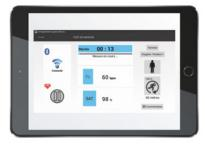
Real-time display During test, the software displays and records, in real time, oxygen saturation and heart rate.
